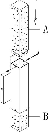
Install the crystal A.B. to the relevant position of the lamp body.
